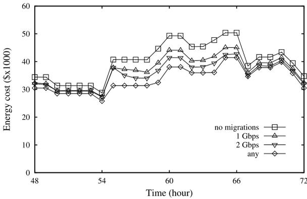
Fig. 14. Total energy cost per hour vs. time during the third day after the initial assignment, with different allowed migration rates.
