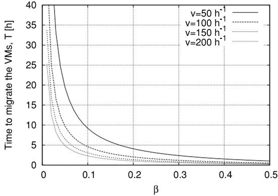
Fig. 6. Time to migrate the VMs versus  $\beta$ , for several values of the migration speed,  $\Delta C = 0.2$   $\$/kWh$ .
