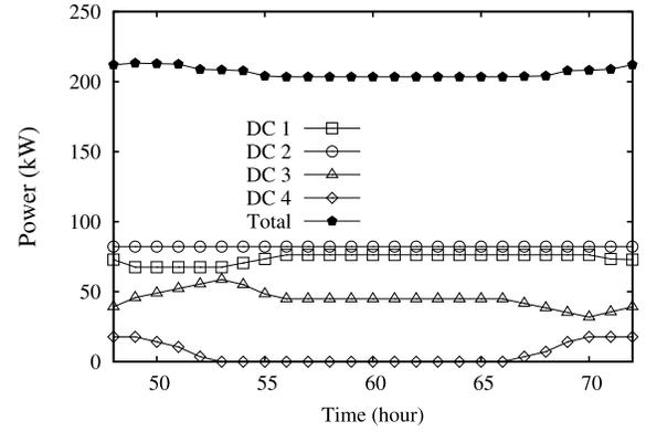
Fig. 19. Power consumption of DCs vs. time during the third day after the initial assignment, with  $\beta=0$ . Overall load  $\Lambda=50\%$ .
