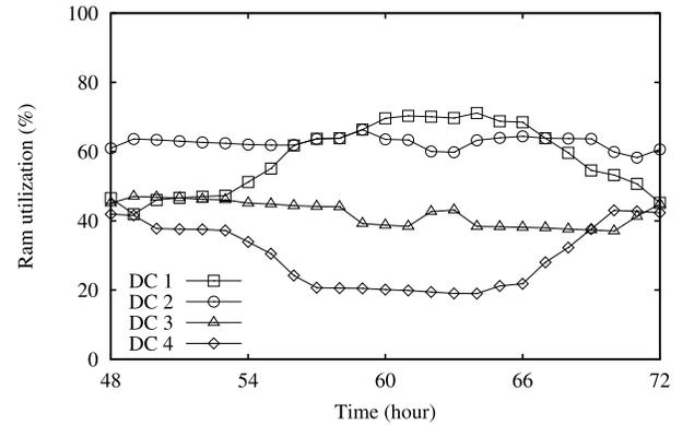
Fig. 12. Utilization of DCs vs. time during the third day after the initial assignment.
