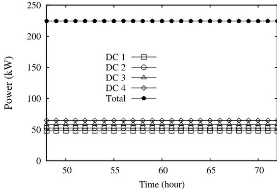
Fig. 18. Power consumption of DCs vs. time during the third day after the initial assignment, with  $\beta=1$ . Overall load  $\Lambda=50\%$ .
