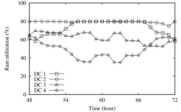
Fig. 17. Utilization of DCs vs. time during the third day after the initial assignment. Overall load  $\Lambda=75\%$ .
