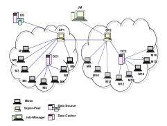
Fig. 3. Network architecture for the MINING@HOME experiments
